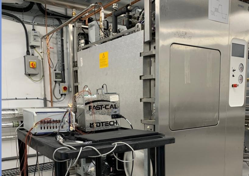
Decontamination of re-useable surgical instruments is classified as re-manufacturing under the Medical Devices Directive. The Directive is harmonised with equipment technical standards covering, EN 285:2015 details best practice for Steam sterilizers and for Washer Disinfectors EN / ISO 15883-1:2009 applies, Part 1 covers General requirements, terms and definitions and tests.
