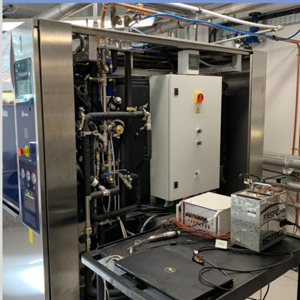
The Isotech Fast-Cal temperature reference source, or dry block, is ideal to validate the thermocouples before and after the validation process.
