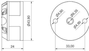
Mounting holes: two holes 4.9 mm diameter, 33 mm centres.
