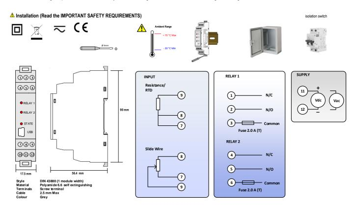
Input connections for cable length >3 metres use screen or twisted pair cables. PT100 connection all wires must be equal length (resistance). Maximum cable run 30 metres.
