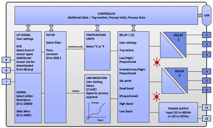
⚠ Configuration (Read the IMPORTANT SAFETY REQUIREMENTS) During configuration the equipment takes its power from the USB port, therefore no power connection is required. The equipment can be configured whilst powered but the computer used must be isolated from the supply earth to avoid grounded earth loop effects. Refer to configuration help guide for further information on configuration methods.
