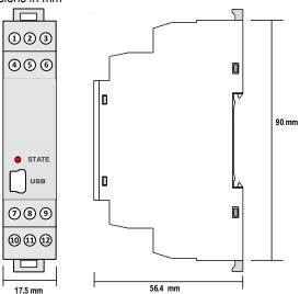
The equipment must be mounted on a DIN rail style DIN EN50022 inside a plastic or metal enclosure with a protection level >= IP65. All wiring must be secured. Maximum cable sizes 2.5 mm<sup>2</sup>. Connection is via screw clamp terminals.
