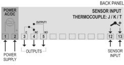
Figure 5 – Connections (Thermocouple)
