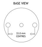
Fixing holes 2 x Ø5.5 mm, Centre hole Ø4.5 mm
