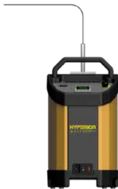
A control system with digital display shows the set and measured value from the calibration volume.
